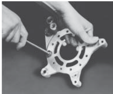
Handles generally used with radius deburr tools. For other shanks, see pages 78-80.
