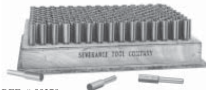
REF. # 55378 Severance can do either small or large runs on special tools. Such as these Midget Mills® with a special cut.
